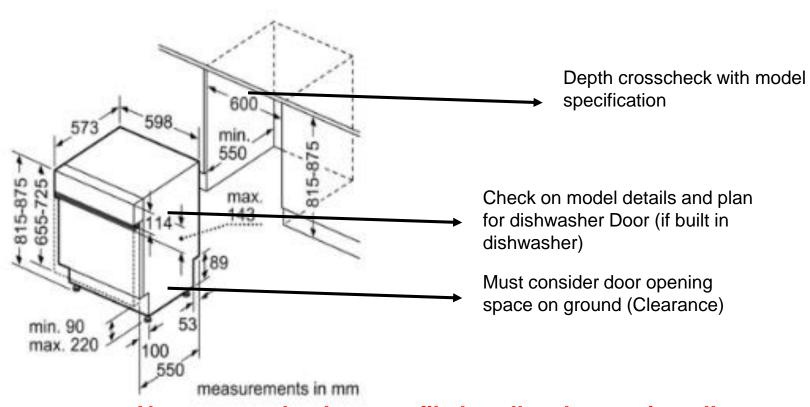
Note: crosscheck on profile handles, how to install
