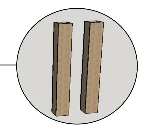
NOTE: The clear space between the pillars should be minimum of 100mm.
